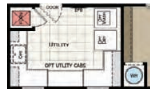
Utility room layout for Multi-Section only
